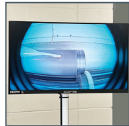
Camera and viewing monitor allow visibility without stopping machine
