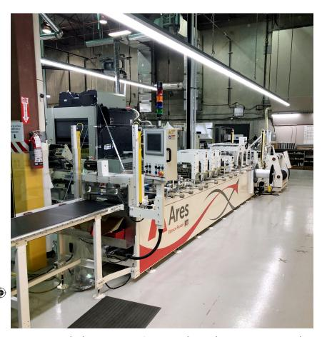
With the Ares 400 SUP pouch machine at Associated Labels and Packaging, one operator selects the recipe and does all the packing duties for the line. Image courtesy of Associated Labels
